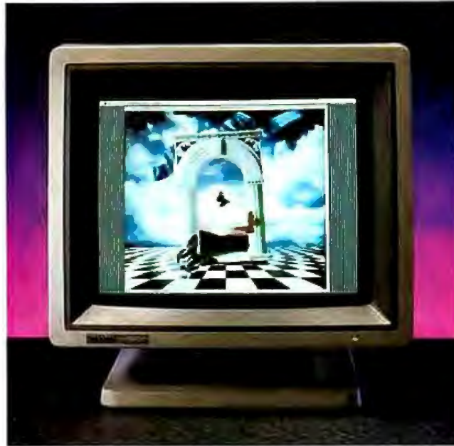
Taxan's Ultra Vision 1000 monitor reaches scan rates of 78 kHz.
