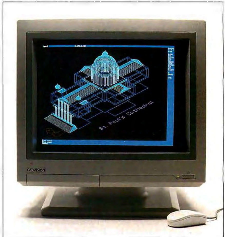
Photo 2: The Chugai Cadvision offered good resolution but was not multisyncing. It's best suited for CAD applications.
