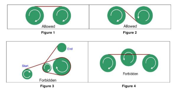
One task in setting up such mechanical systems is to link together two given shafts, subject to these constraints:
