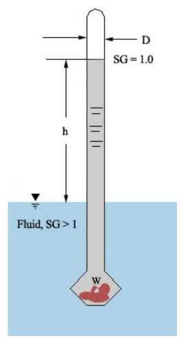
Figure 1 : A Hydrometer
