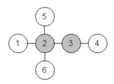
Move obstacle 2-5, then 3-2-6, and then move the robot 1-2-3-4. Total: 6 moves.
