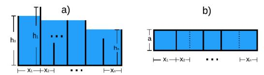
a) Frontal view of the tank. b) Aereal view of the tank (Dotted lines are submerged walls)
