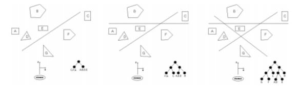
Assuming you have split the partitions correctly, a simple traversal of the BSP tree will give you an appropriate ordering for which to render the objects in the scene. Note in the example above that once a node contains just one object it need not be split as additional planes are added.
