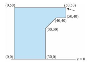
Figure C.1: Crane cross section
