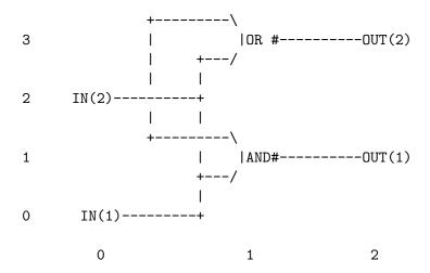
In grid terms this is two inputs at 0,0 and 1,0. The first input feeds the AND operation at 1,1 and the OR operation at 1,3. The second input operation feeds the second input for the same AND and OR operations. The AND operation then feeds an output operation at 2,1. The OR operation also feeds an output operation, this one at 2,4.
